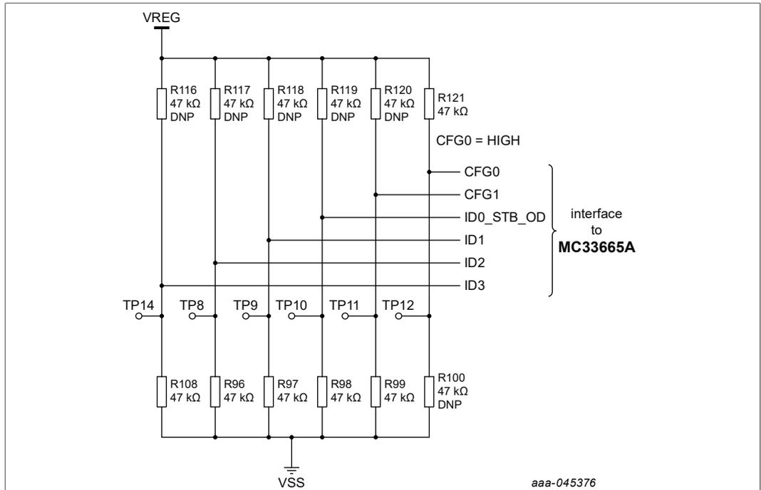
Figure 4. CAN HW settings for MC33665A
