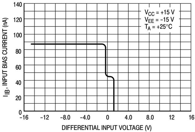
**Figure 5. Input Bias Current versus Differential Input Voltage**
