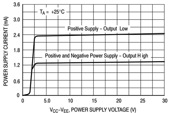
**Figure 14. Power Supply Current versus Supply Voltage**
