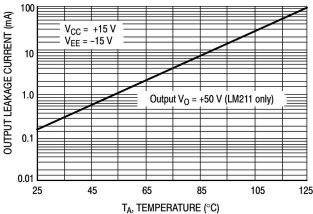
**Figure 13. Output Leakage Current versus Temperature**
