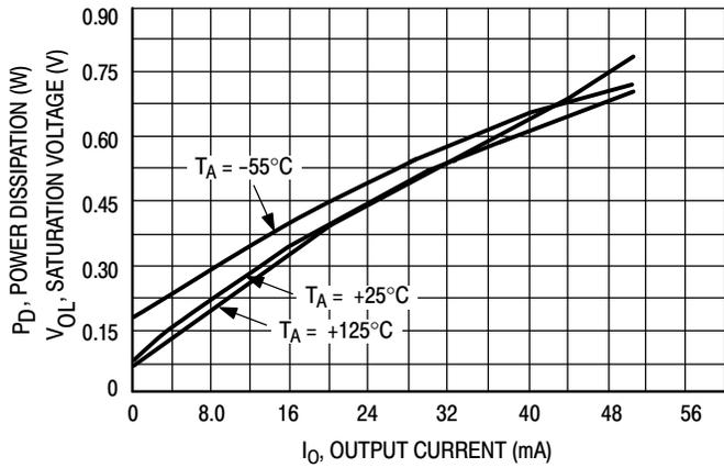
**Figure 12. Output Saturation Voltage versus Output Current**
