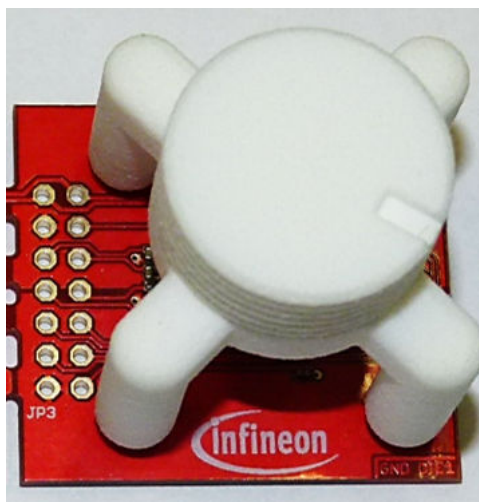
Figure 2 Rotation knob with TLE5x09A16(D) angle sensor below
